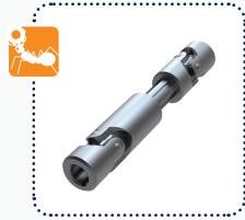
R3680 Telescopic Universal Joints 9SMnPb28k, no.10718, greased. To DIN 808
