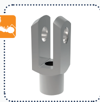
R3385 Clevis Joints 1.0718 (11SMnPb30k), silver zinc plated
