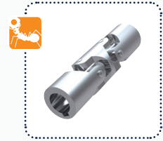
R3685 Double Universal Joints 9SMnPb28k, no. 10718. To DIN 808
